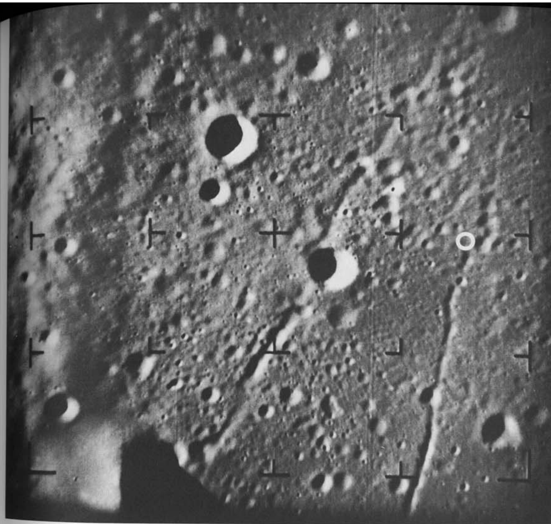
FIGURE 31. The first six craters in order of size shown here can be identified readily as small pits in Fig. 26, located within three impact-circle diameters of that circle. Note the great number of craters shown here in areas that appear smooth in Fig. 26 and later pictures. The two prominent rills are disintegrating into chains of craters and shallow depressions as resolution continues to increase. Two general classes of craters are now evident: sharp, round, deep ones and soft, shallow ones. Some of the latter are irregular in outline. Ranger 9's altitude is 35.1 miles 23.5 seconds before impact. Picture width is 16.2 miles.
